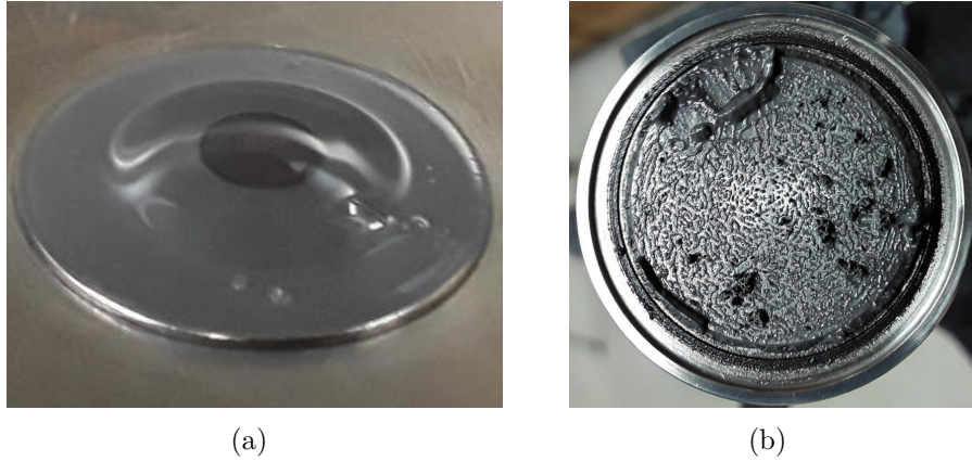
Figure 4.8: Fluid after rheometer testing with (a) the field off (b) the field on
