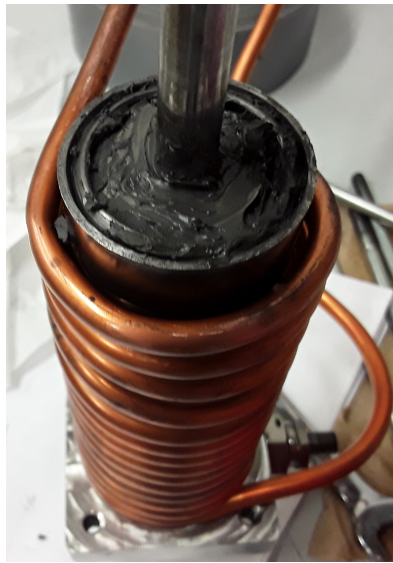
Figure 4.14: Damper and piston after endurance testing
