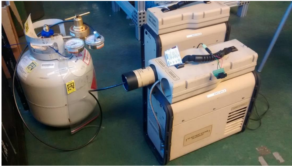
Figure 45: Two Ultra/AMI D300 APUs with standard propane tank supply
