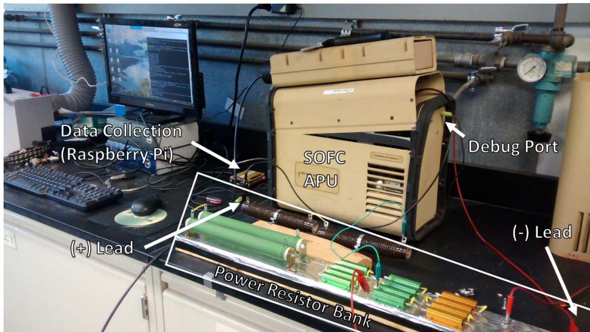
Figure 48: Image of SOFC APU experimental setup
