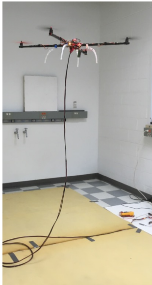
Figure 5.1: Quadcopter flight test with electrical tether for power delivery.
