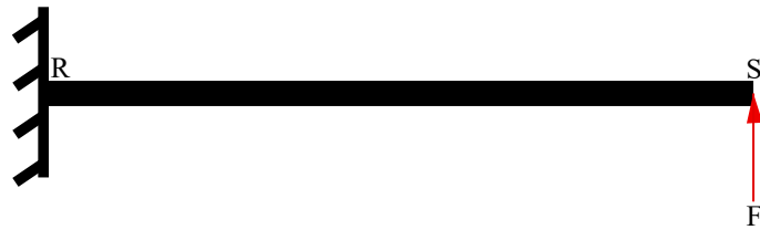
Fig. 5.7: Tip loaded cantilever beam modelled in Dymore.
