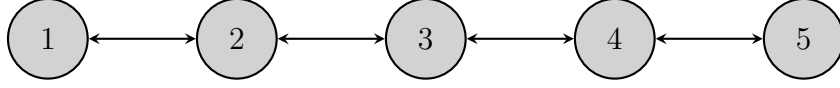
Figure 3.6: Communication graph for the 5 agents controlling the nonlinear system. This graph has the structure of a path which is a type of tree.
