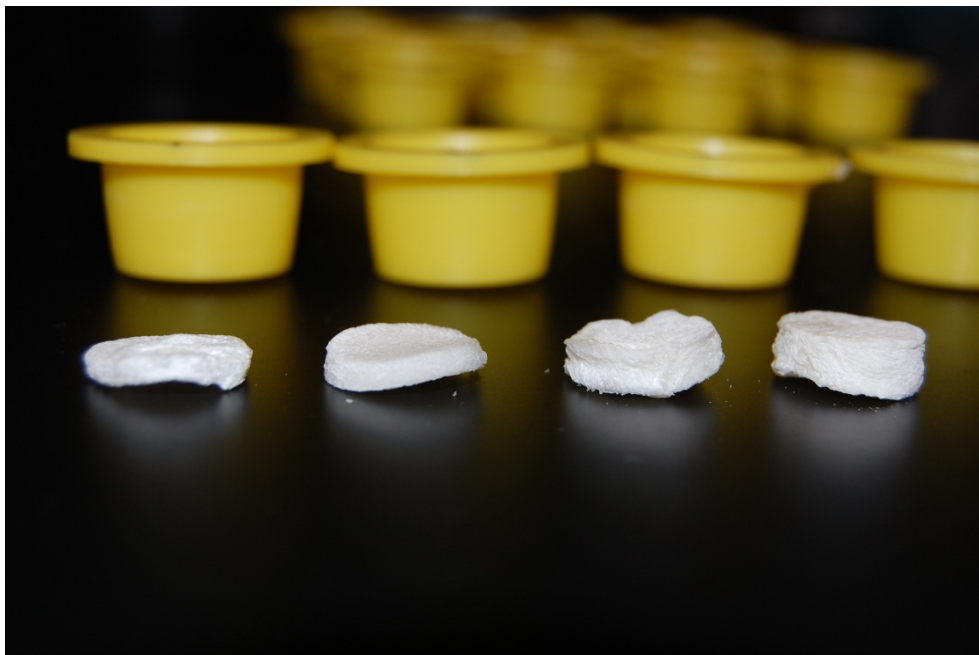
Figure 37. Calcium cross-linked ASD prepared from 2% alginate and fill volumes ranging from 1-4mL (left to right). Note the brilliant white appearance and warped morphology after being cross-linked and lyophilized a second time.
