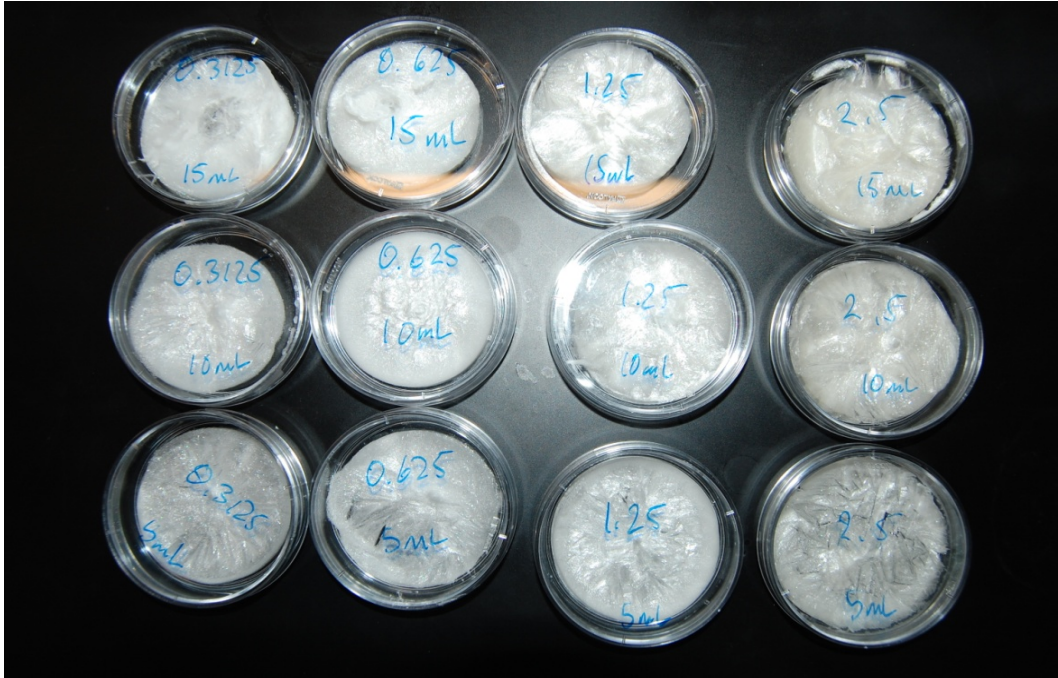
Figure 33. ASD prepared from alginate concentrations 0.3-2.5%, and fill volumes ranging from 5-15 mL. ASD prepared with 0.3% alginate solutions and low fill volumes of less than 10 mL were often delicate and contained numerous large cracks.
