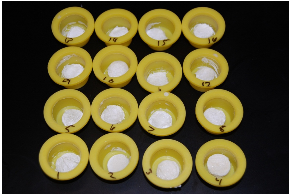
Figure 36. Dry ASD cross-linked with calcium. Samples 1-4, 5-6, 9-12 and 13-16 were prepared from 2, 1, 0.5 and 0.25% alginate solutions and fill volumes of 1-4mL respectively.
