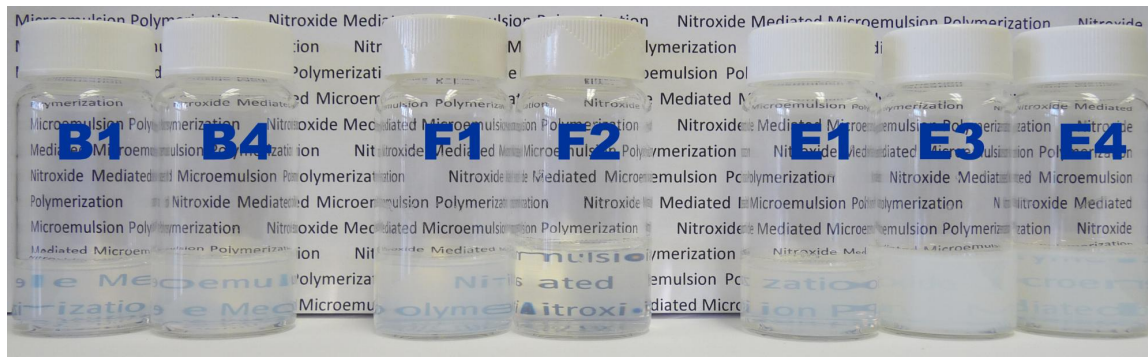
Figure 6.14: Selected microemulsion latexes: 17% solids both with 8 mol% and 30 mol% St in the 1 st stage (B1, B4), (MMA-co-St)-block(BMA-co-St) latex (F1), (BMA-co-St)-block(MMA-co-St) latex (F2) and 40% solids latexes (E1, E3 and E4).
