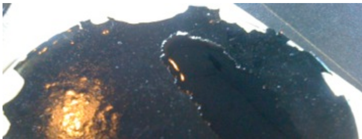
Figure 4.2: Representative bulk film of 20 % (w/w) PANI-loaded PDMS. Significant tearing and crumbling of the sample is apparent along the film edges.
