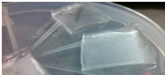
Figure 4.1: Representative bulk unloaded PDMS films. PDMS to heat cure ratios of 5:1 and 10:1. No visual difference observed.
