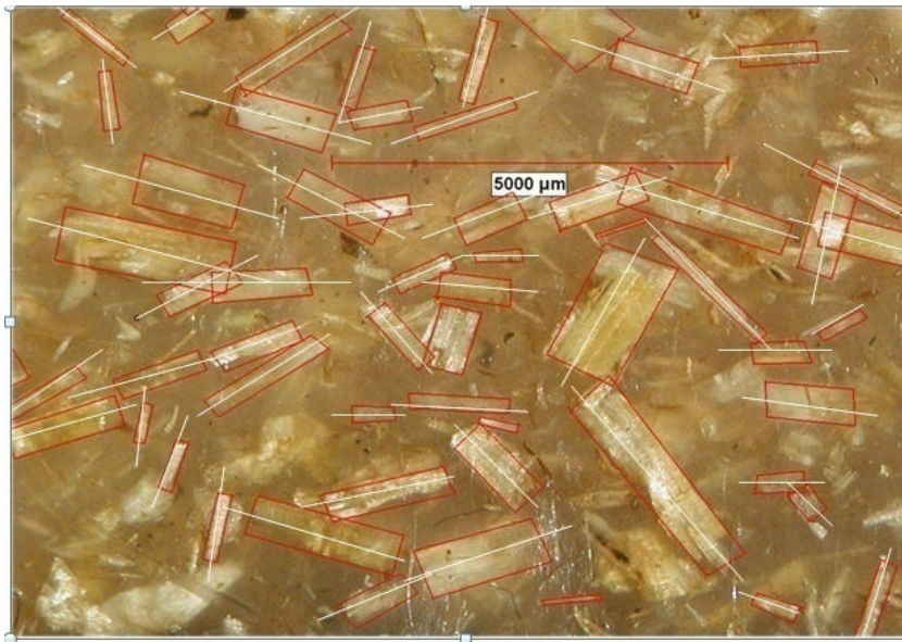
Figure 7.10 The milled wheat particles on the surface of the composite approximated as rectangles with axial lines
