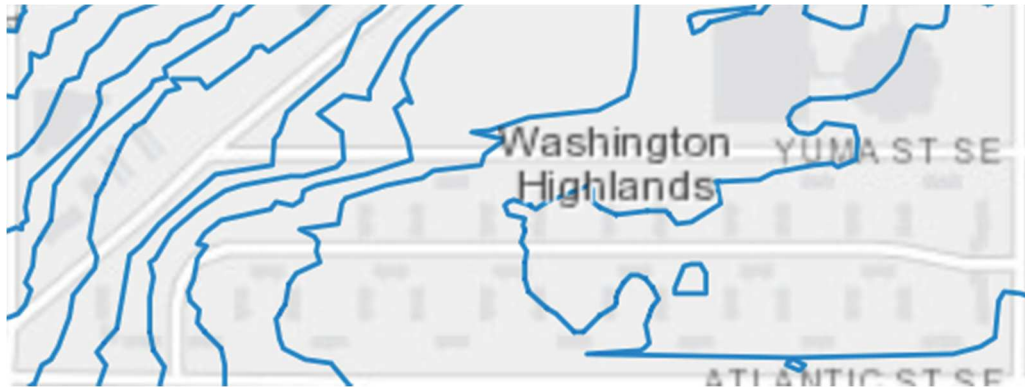
Topographical map of the Washington Highlands complex. The blue lines represent ten-foot changes in elevation from the highest points on the right to the lowest to the left. Screenshot taken from the District of Columbia Geographic Information System, “Topography-10 Foot Contours,” courtesy of the District of Columbia Open Data Project, https://opendata.dc.gov/datasets/topography-10-foot-contours?geometry=-77.006%2C38.830%2C-76.991%2C38.833 (accessed November 29 th , 2019).
