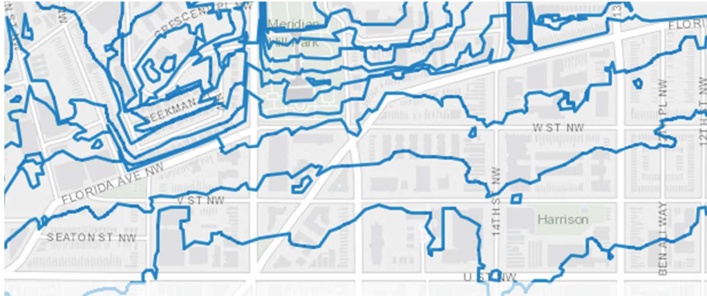
A topographical map of Washington with Florida Avenue NW labeled in the middle of the image. The map contours represent ten-foot changes in elevation. Note how north of Florida Avenue the elevation increases dramatically. Map acquired from Open Data D.C., “Topography - 10 Foot Contours,” https://opendata.dc.gov/datasets/topography-10-foot-contours (accessed January 11 th , 2020).
