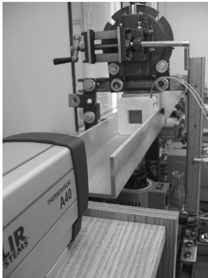
Figure 27: Photograph of the partially disassembled experimental heat exchange apparatus used in this work, with a view of the FLIR system, the clamping mechanism, a prototype insulation block and heating controls.
