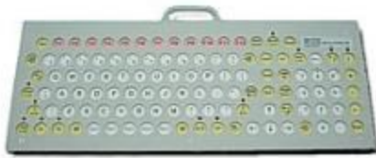
Figure 2.1: A keyboard with raised areas between keys for users with tremors or spastic movements [60].
