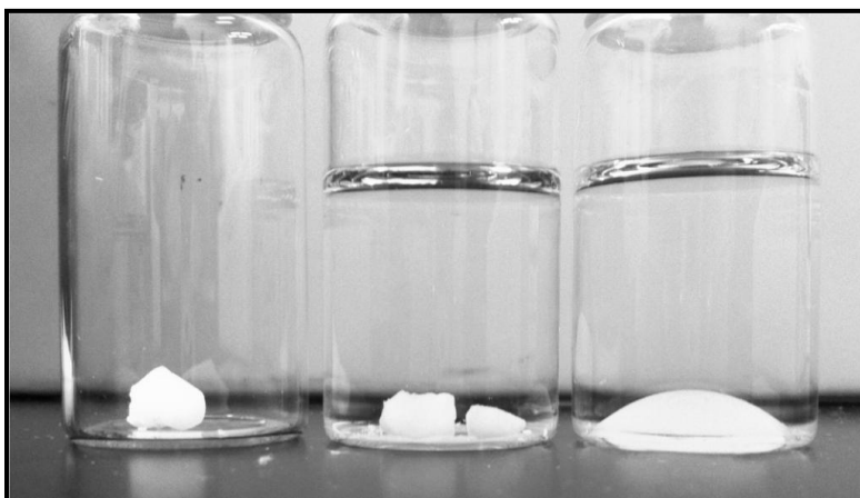
Figure 10 - PTMG (2.9 kg/mol) as-received (left) and after soaking in pure water (centre) and in a n -butyric acid solution (2 wt%) (right)
