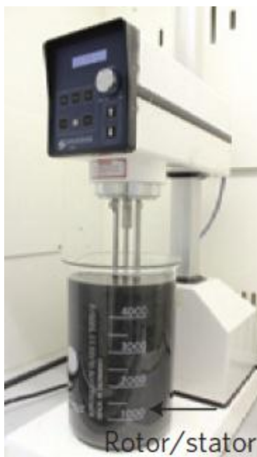
Figure 2.8: A Silverson high-shear mixer (Model: L5M-A) exfoliating a graphite dispersion [58].
