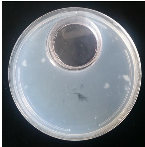
Figure 3.2: An injection stage, with a 35 x10 mm dish acting as microparticle reservoir, for positioning anesthetized embryos during microparticle injection.
