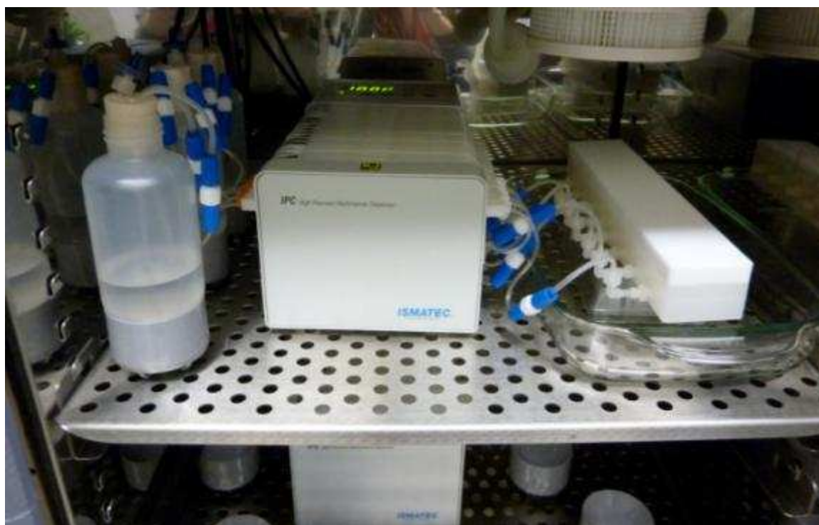
Figure A 1 Set-up of the continuous flow bioreactor housed within the incubator
