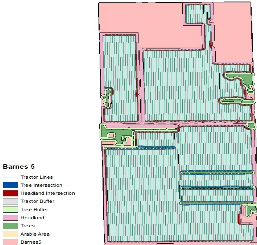
Figure 12. Simulation of Tractor Lines, Intersections around Headland and Non-Navigable Obstacles
