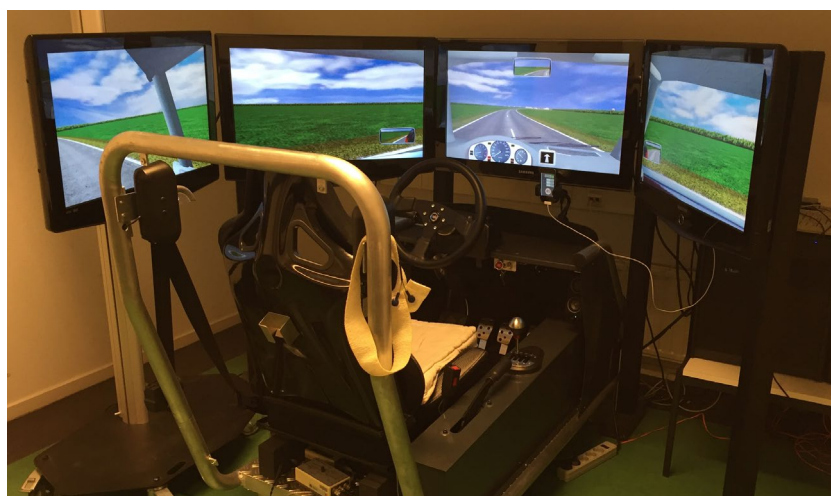
Figure 1. The Groningen driving simulator, with the UBI device (the iPod) mounted on the simulator frame.
