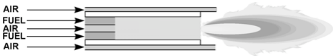
Figure 2.13: Schematic Diagram Depicting a Partially Premix Burner (Baukal, 2000)
