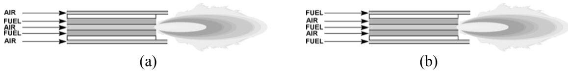
Figure 2.18: Schematic Diagrams Depicting (a) Staged-air Burner and (b) Staged-fuel Burner (Baukal, 2000)
