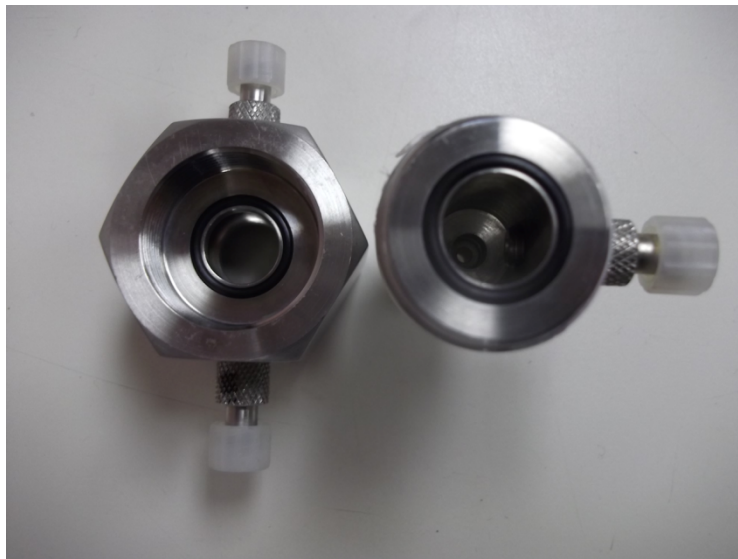
Figure 3-3. Mid-chamber (left) and main chamber (right) that comprise the hydrostatic pressure chamber.
