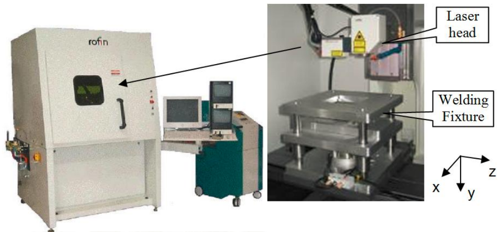
Figure 4-1 Rofin-Sinar DLx16 HP diode laser and welding fixture in UW200 Workstation [41]
