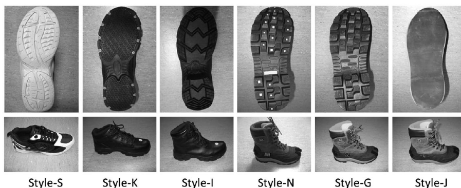
Figure 1. Test footwear. Six styles of footwear were selected for testing including a running shoe (Style-S), an indoor slip-resistant boot (Style-K) and four winter boots.
