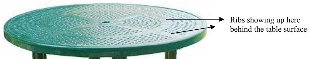
Figure 2-5 An example of hiding the sink marks using the surface texture
