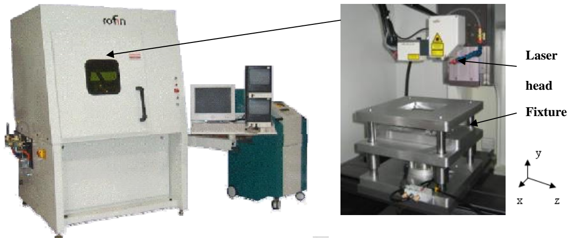
Figure 4-1 Rofin-Sinar diode laser cabinet (left) and close-up view of the DLx16 laser head and the welding fixture (right).
