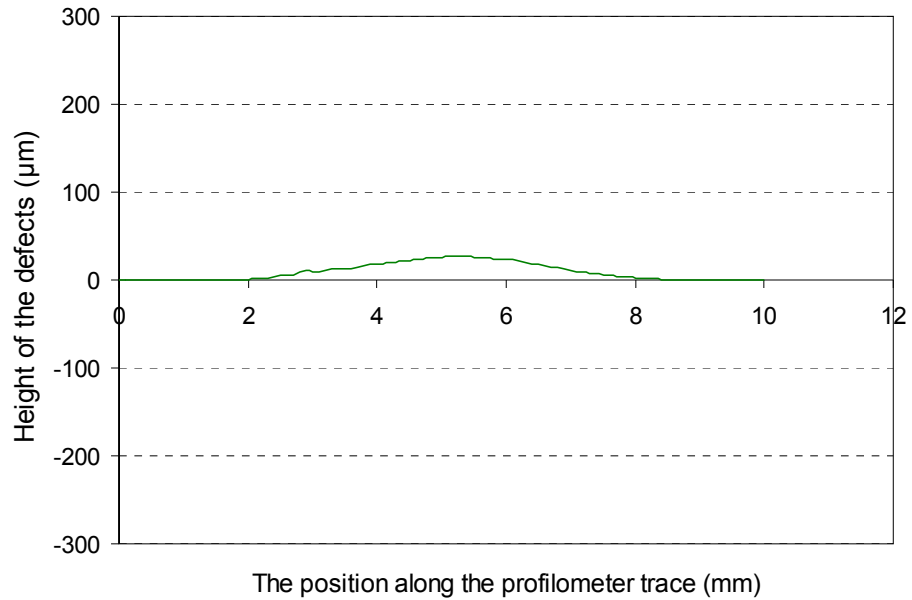
Figure 4-15 A typical shape of ribs obtained using the method in Section 4.2. This data is for a 2 mm thick part containing a CB level of 0.05 wt. % and welded at a power of 18 W (this defect was created near the beginning of the “weld seam”)
