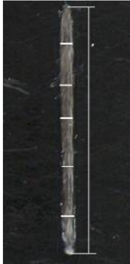
Figure 6-3 Weld width and length measurement on the fracture surface after the shear strength test
