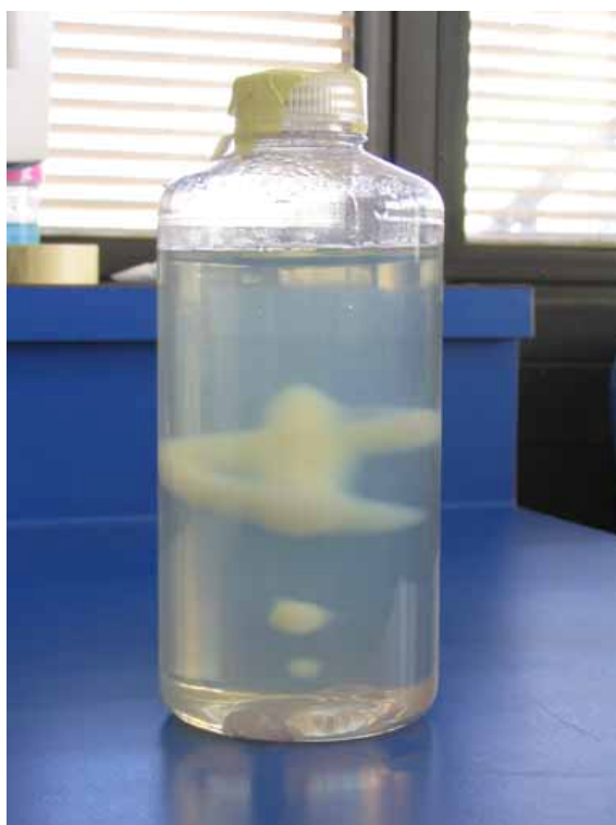
Figure 2.3: Photograph of a non-uniformly irradiated polymer gel dosimeter phantom of approximately 1 L. The white regions, which received higher radiation dose, contain more precipitated polymer than the surrounding transparent gel.
