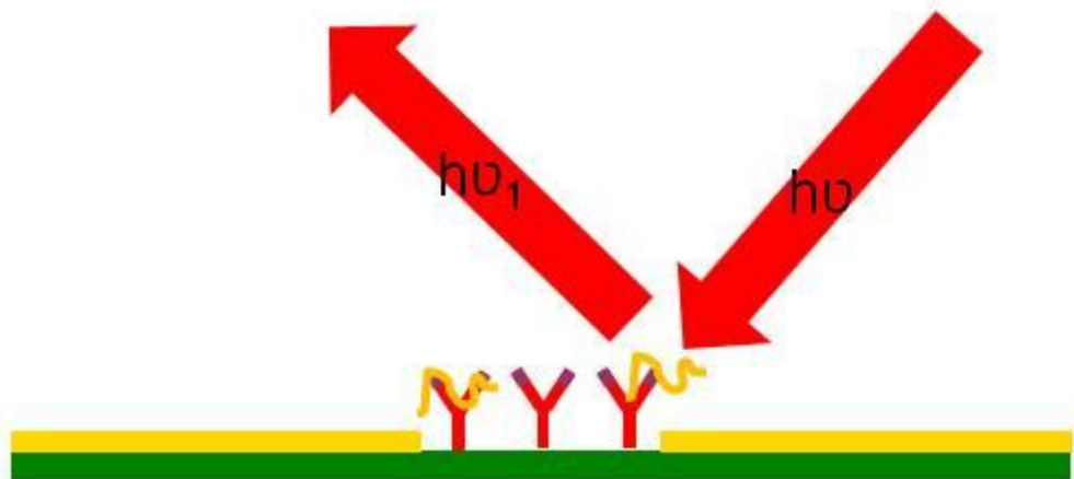
Figure 41: Proposed scheme for Raman spectroscopy coupled with an AC electrokinetically enhanced surface based biosensor. Gold microelectrodes (yellow) on an antibody (red “Y” shaped molecules) functionalized silicon substrate (green) with positive dielectrophoretically attracted viruses (orange wavy lines). A laser with a known energy ( h\nu ) is directed towards an area containing viruses and the resulting Raman spectrum of the shifted light ( h\nu_1 ) is recorded.
