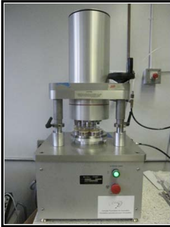
Figure 4.1 The AMTI Ortho-Pod ™ six station pin on disc friction and wear testing machine.
