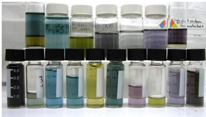
Figure 7: Monodisperse SWCNT solutions demonstrate a striking array of colors. Blue solutions are metallic SWCNT enriched, (6,5) enrichment bring out the color purple, and (7,4) enrichment is responsible for yellow. 48,49
