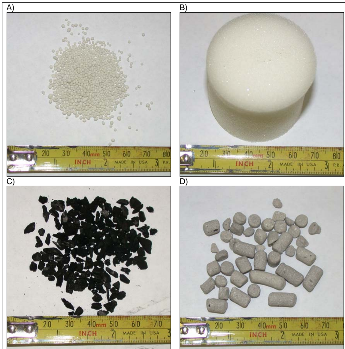
Figure 3.2: Photographs of carrier materials (ruler for scale). A) Poraver™ porous glass beads; B) polyurethane foam plug; C) bone char; D) Celite™ R-635 diatomaceous earth pellets.
