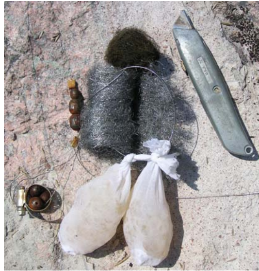
Figure 3-3: Photo of steel wool and nutrient bundles before being put down well.
