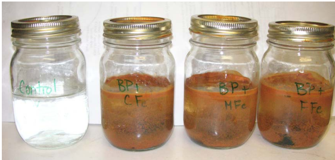
Figure 3-2: Photo of 3 jars containing nutrient and steel wool, and the one control jar.
