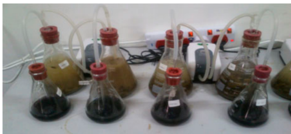
Figure 1. Ammonia volatilization forced-draft set-up.
