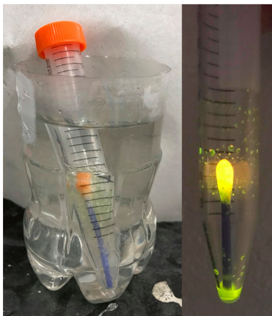
Figure 2. (Left) Liquid CO 2 extraction of dyes contained in orange glow stick fluid. Note the slight yellow tint of the liquid CO 2 that surrounds the cotton swab. (Right) Cotton swab and extract after extraction procedure and warmed to room temperature.
