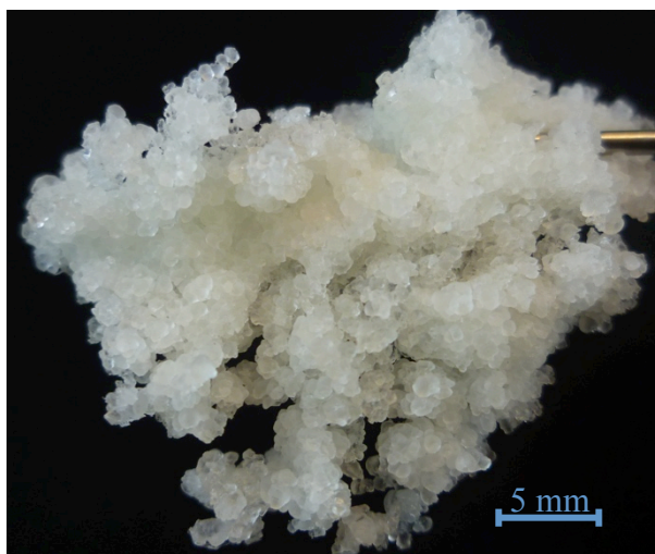
Figure 5.2. Photograph of the coagulated BA/MMA copolymer. The sample was destabilized with air and heat (80 °C).
