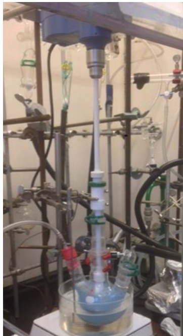
Figure 4.1. Experimental setup, utilising the overhead stirring device, for SI-AGET-ATRP for the synthesis of CO 2 -responsive polymer-grafted spherical silica particles.
