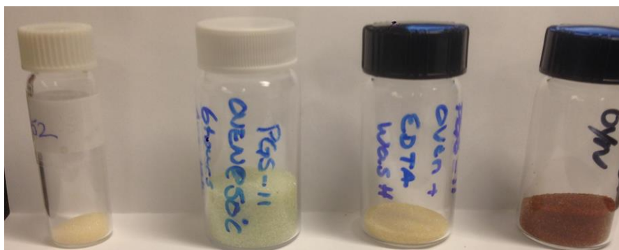
Figure AIII.1. The colours of PGS-11 at various stages of synthesis. From left: initiator-grafted SiO 2 ; PGS-11 as collected; PGS-11 rinsed then dried followed by a wash with an EDTA solution; PGS-11 left overnight in the oven at 110 °C.
