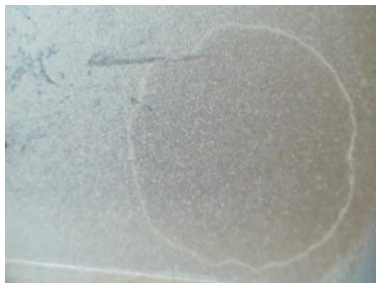
Figure 4.15: Top view of the FSNP surface following exposure to 100% methanol.
