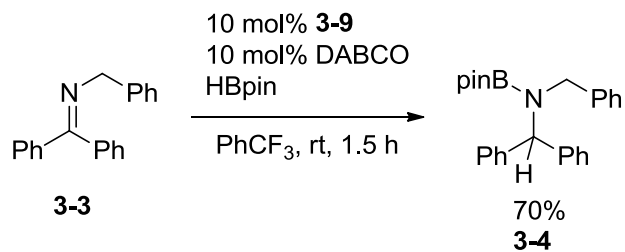
Scheme 3.3-12: Use of 3-9 as an initiator and DABCO as a catalyst in the hydroboration of imine 3-3 .
