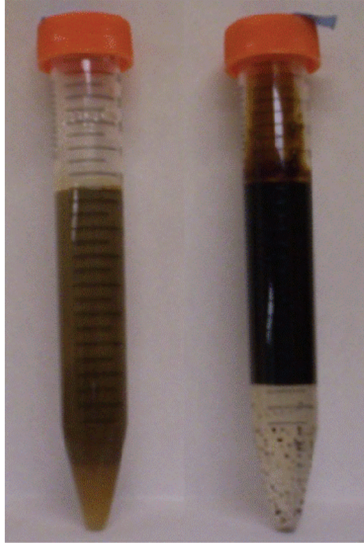
Figure 20 – O/W emulsion of crude oil Sample III in water. Samples untreated after emulsification [LEFT] and treated with CO 2 [RIGHT]. Photographs were taken after four weeks at room temperature.
