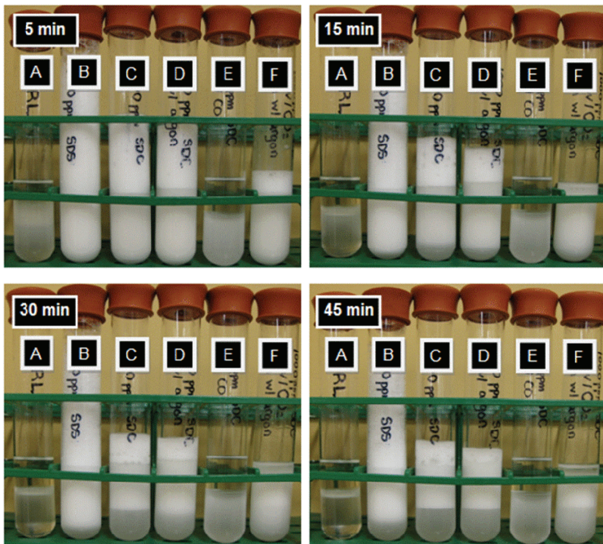
Figure 35 – Phase separation of n-heptane water emulsions. Addition of carbon dioxide caused the emulsion stabilized by sodium laurate to separate immediately, leaving a clear organic layer.
