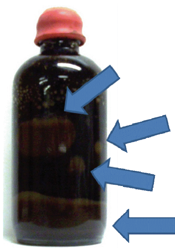
Figure 17 – Water separation after CO 2 treatment of an O/W emulsion stabilized with naturally occurring surfactants activated with Na 2 CO 3 . Water pockets trapped in the heavy viscosity separated crude oil are indicated by arrows.
