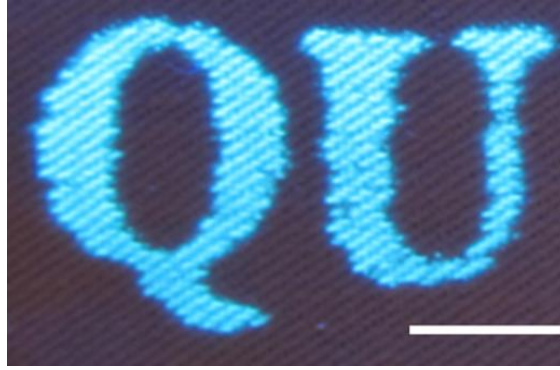
Figure 2.18 Fluorescent pattern of “QU” that had been printed using an aqueous PEO-Py solution as the ink onto cotton fabric. The scale bar represents 1.0 cm.
