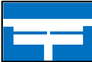
Figure 3-5 Pattern scheme of ITO glass slide. The blue part is covered by tape so that the ITO layer remains, the white part is uncovered glass.
