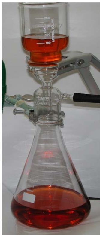
Figure 4.1 Filtration apparatus used to remove proteins from sample solutions. 3M Empore C 8 or C 18 extraction disks were used for the filtration. Following the filtration the proteins were extracted from the disk and analyzed via MALDI-MS.
