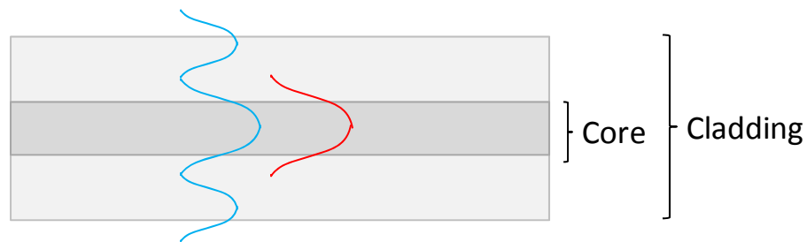
Figure 1.5 Core propagating mode (red) and a cladding mode (blue) travelling through a single mode optical fiber. The curves for each mode represent the variation in light intensity across the fiber.
