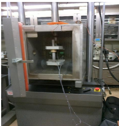
Figure 3.2.5: Loading Frame and Chamber of Material Testing System (MTS).
