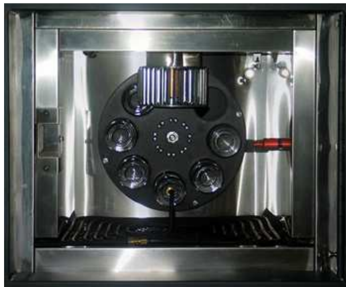
Figure 13. Rolling Thin Film Oven (RTFO) with empty glass jars held inside [10].
