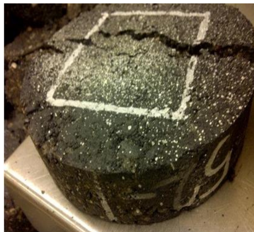
Figure 3.9 Picture of a sample after ITS experiment, showing the painted side used for the digital image correlation (DIC).
