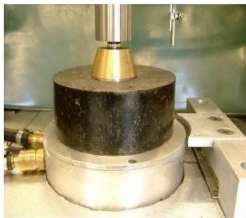
Figure 3.6 Uniaxial cyclic compression test with partial confinement (UCCTC) [53].
