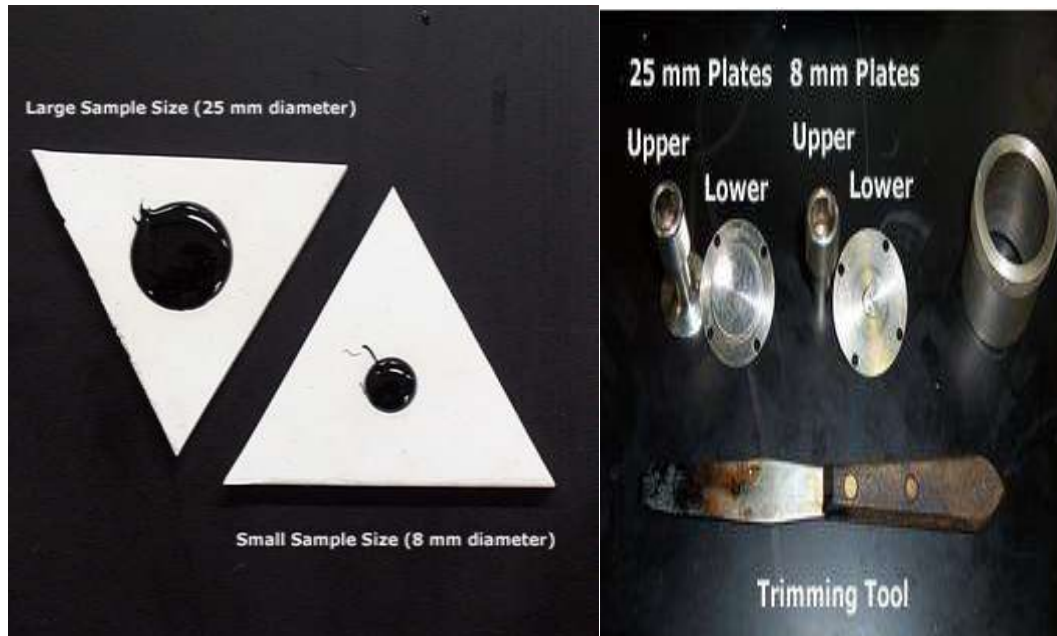
Figure 3.4: (a) DSR sample moulds showing the different sizes and (b) major DSR test tools [64].
