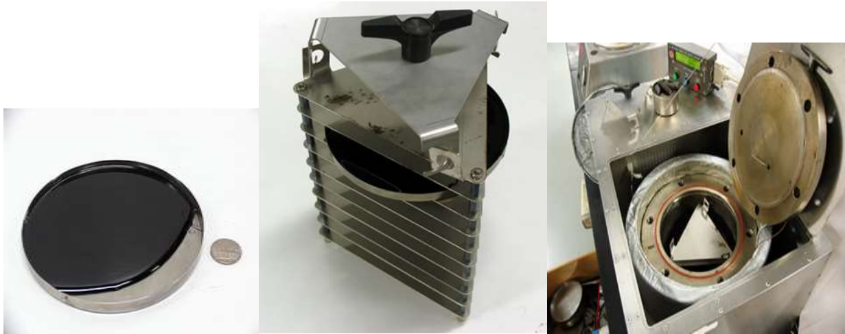
Figure 3.3: Pressure aging components used for long term aging [63].
