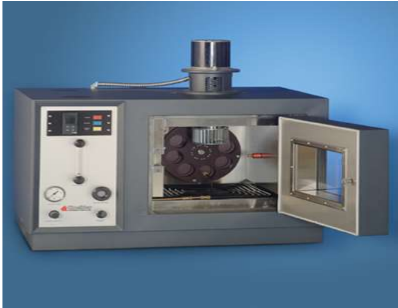
Figure 3.1: Rolling thin film oven (RTFO) used for short-time aging of asphalt binders [61].
