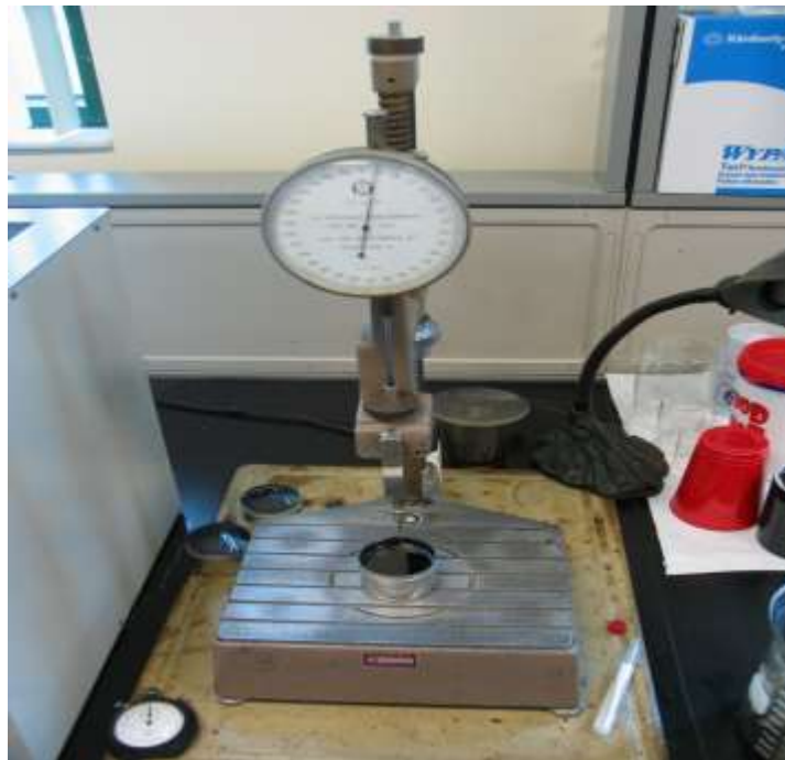
Figure 2.6: Penetration test equipment [34].
