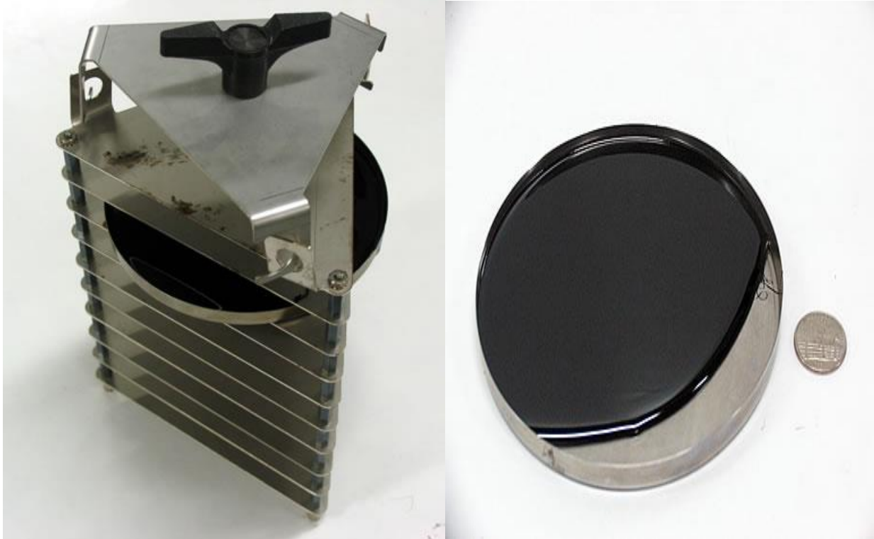
Figure 3.2: Sample preparation for PAV tests [42].
