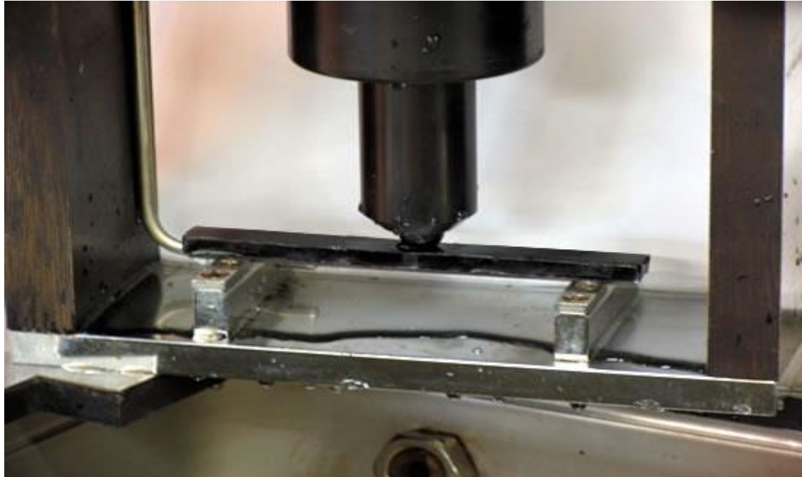
Figure 3.6: BBR beam ready to be tested [46].
