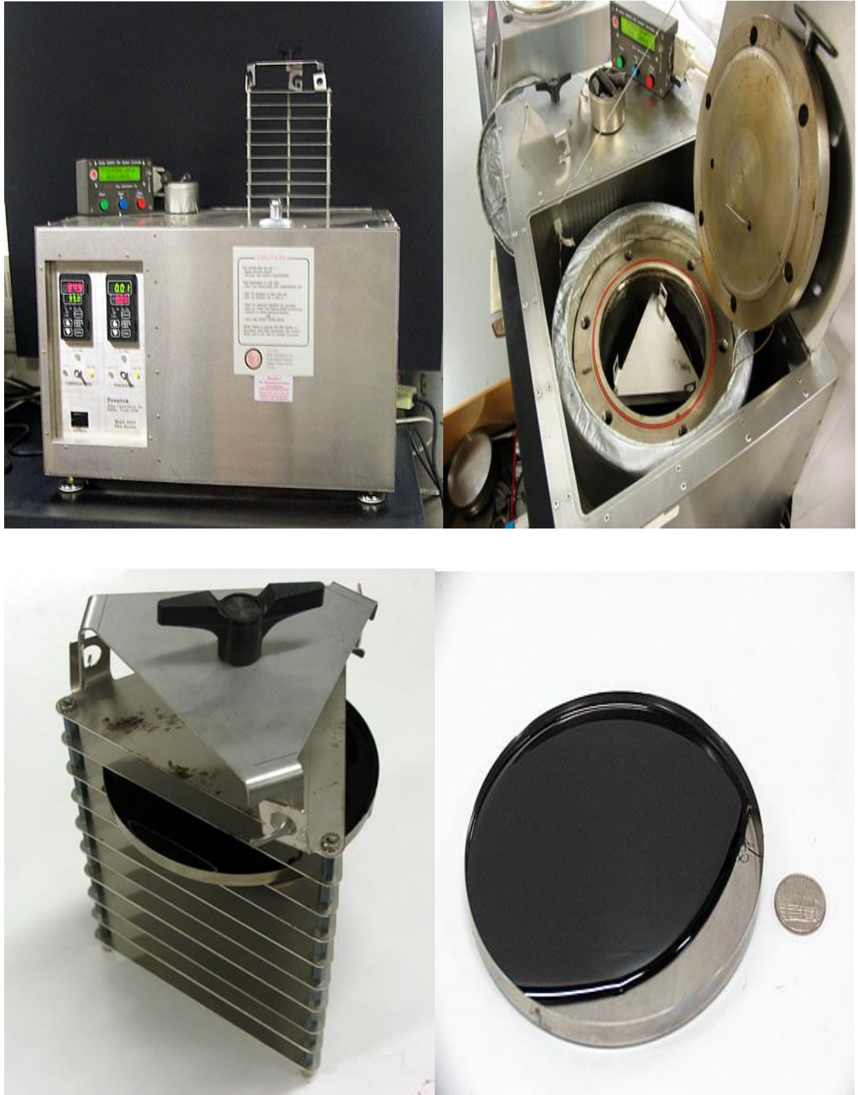
Figure 2.9: Pressure Aging Vessel and its components [42].
