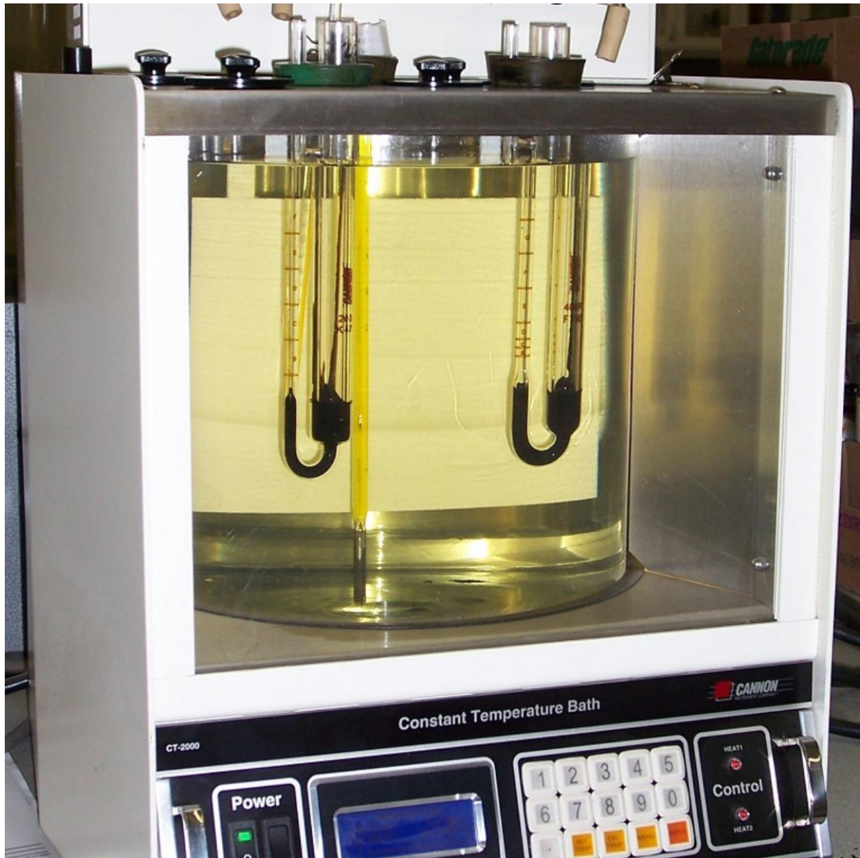
Figure 2.7: Viscosity test apparatus [38].
