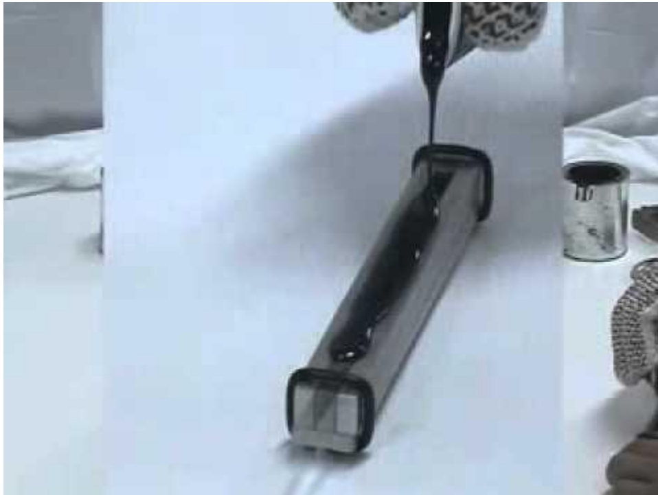
Figure 3.5: Preparation of BBR beams [46].
