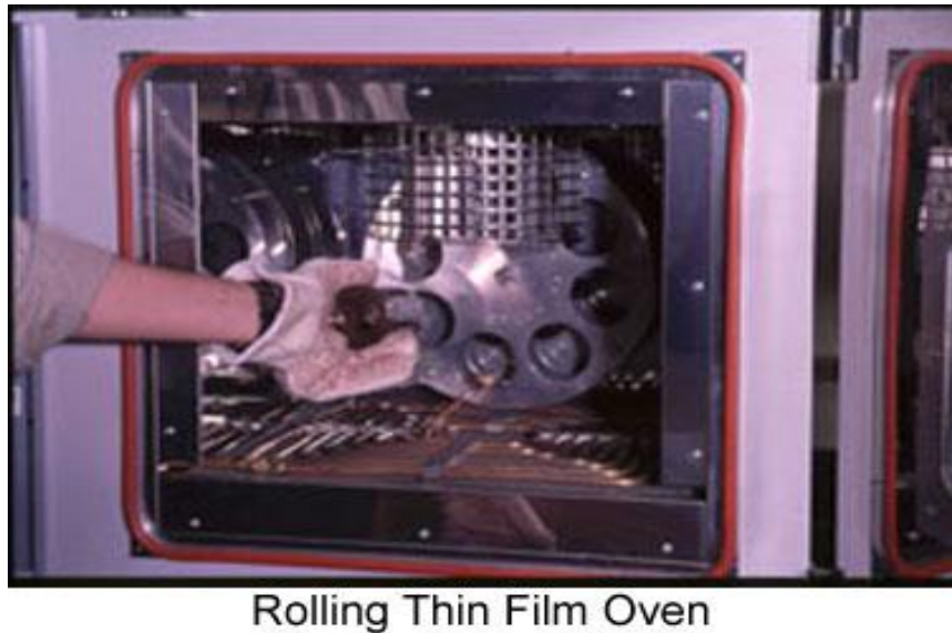
Figure 2.8: Rolling Thin Film Oven (RTFO) [38].
