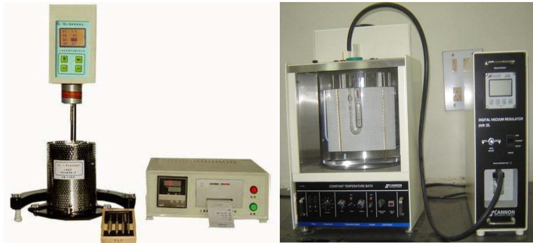
Figure 2.5: Brookfield viscometer [29] and Capillary viscometer [30].
