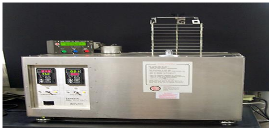
Figure 16. Pressure Aging Vessel [62].
