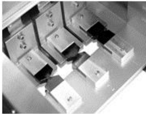
Figure 28. Dent Test Beams Loaded on Testing Pins [68].
