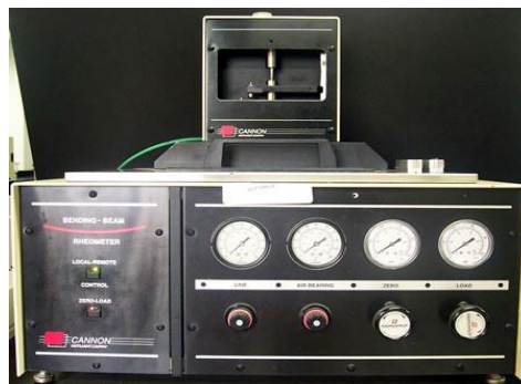
Figure-20. Bending Beam Rheometer [64].
