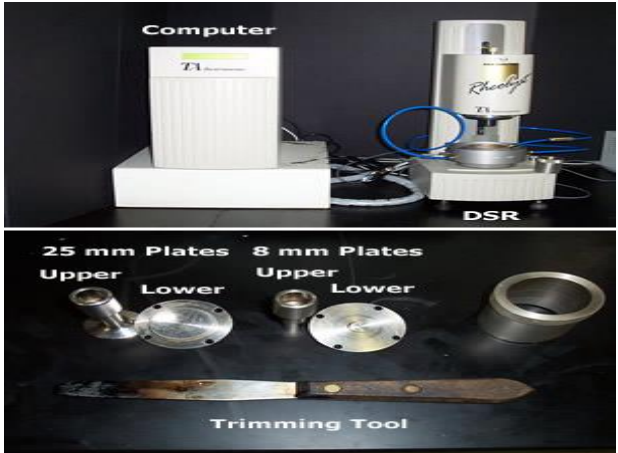
Figure 19. DSR and its components [63].
