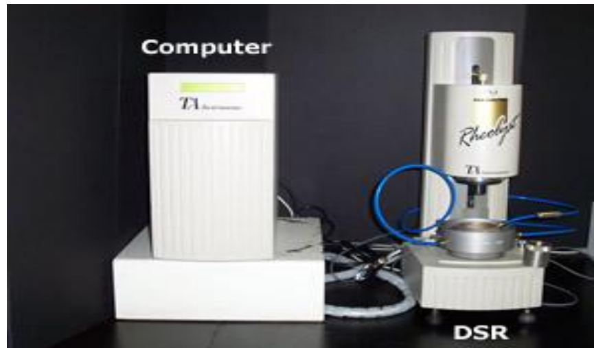
Figure 2.8: Photograph of a dynamic shear rheometer [59].
