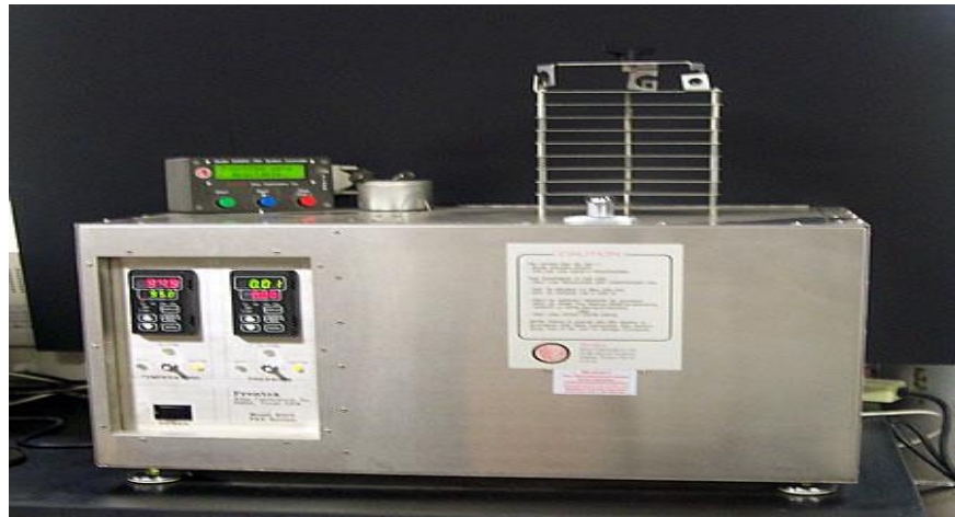
Figure 2.3: Pressure aging vessel for long term aging testing [59].
