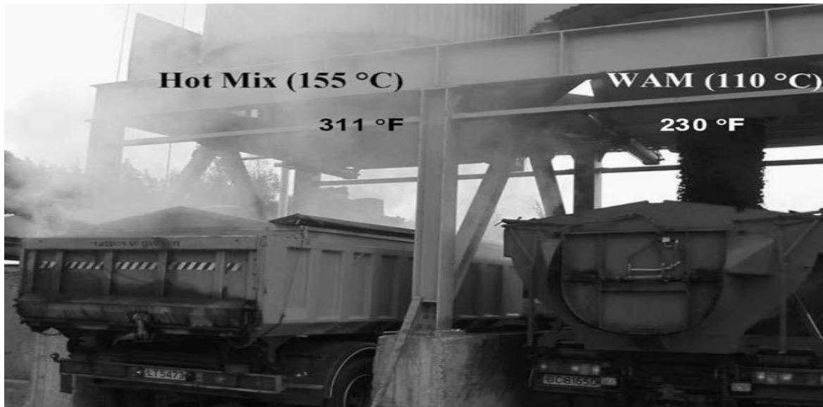
Figure 2.1 Two trucks preparing mix asphalt are side by side, left one containing typical hot-mix asphalt and the right one containing warm mix. It is easily visible that emissions are greater from the hot-mix truck compared to warm mix truck [14].
