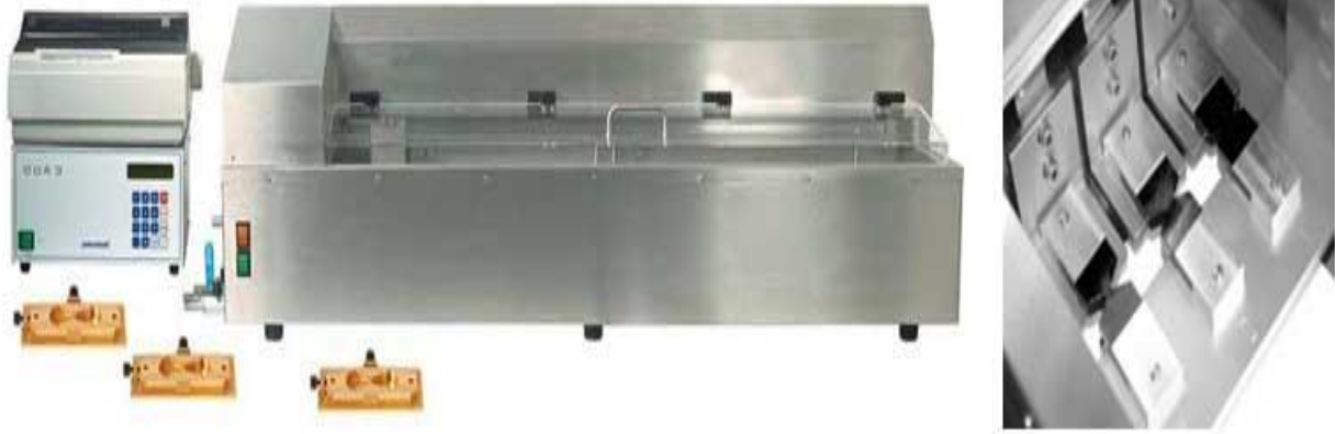
Figure 2.13: DENT test setup [52].
