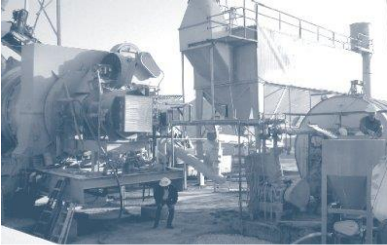
Figure 2.9 Feeder (right) and an existing fibre addition line for Aspha-min® zeolite in Florida [55].
