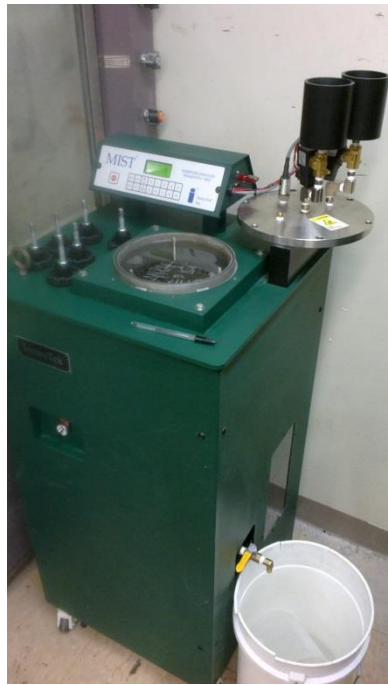
Figure 3.6 MiST conditioning system.
