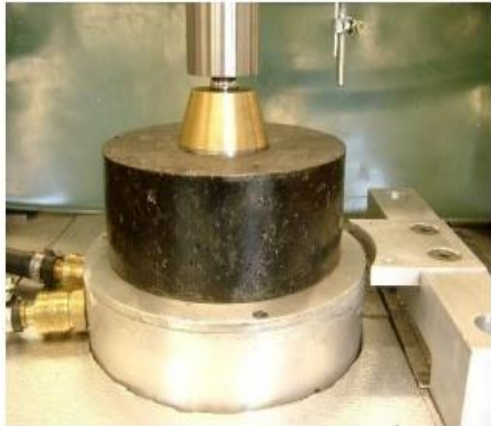
Figure 3.9 Uniaxial Cyclic Compression Test with Partial Confinement (UCCTC) [91].
