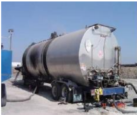
Figure 2.6 Typical blending units for terminal blended projects [49].
