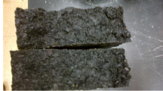
(b) Slight stripping.
